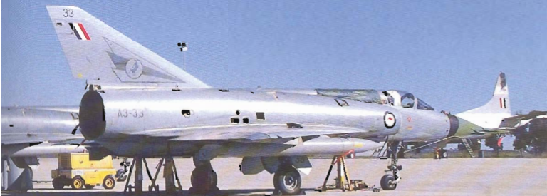
Below Twelve months before it was resprayed, A3-33 is seen heading a line-up of No 75 Sqn aircraft basking in the early morning sun at Pearce Air Force Base in September 1987. Up on jacks, A3-33 is 'Atarless', the squadron groundcrew effecting a quick powerplant change before the day's flying commences (Tony Holmes)
