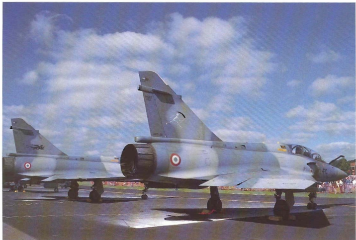
Waving the flag as unofficial NATO members, a pair of Mirage 2000Bs from ECT 2/2 'Côte d'Or' sit side by side on the 40th anniversary ramp at the 1989 Mildenhall Air Fete. From this angle the beefed-up spine associated with the two-seater is clearly visible ( Tony Holmes )
